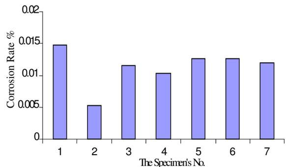
Fig. 2: Corrosion rate in the aquarium
