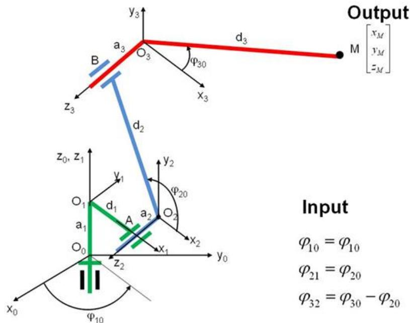
Fig. 1. Geometry and direct kinematics to a MP-3R
