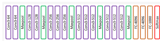
Fig. 3: VGG-16 network presented in Naqvi et al. (2023)
