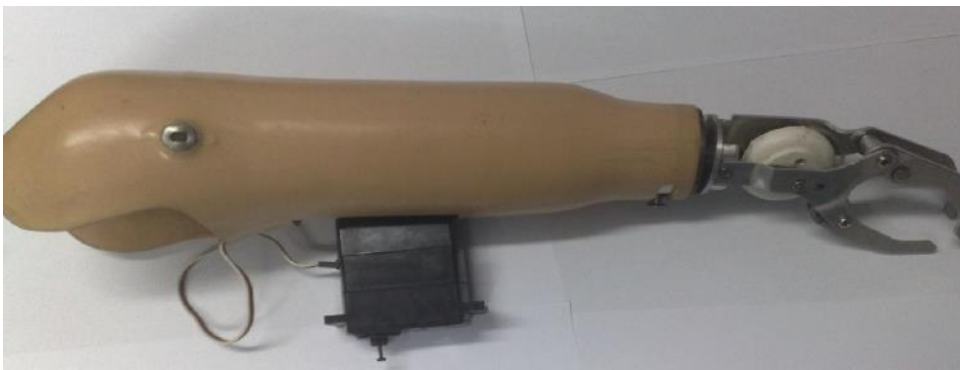
Fig. 6: Final mechanical system of myoelectric arm
